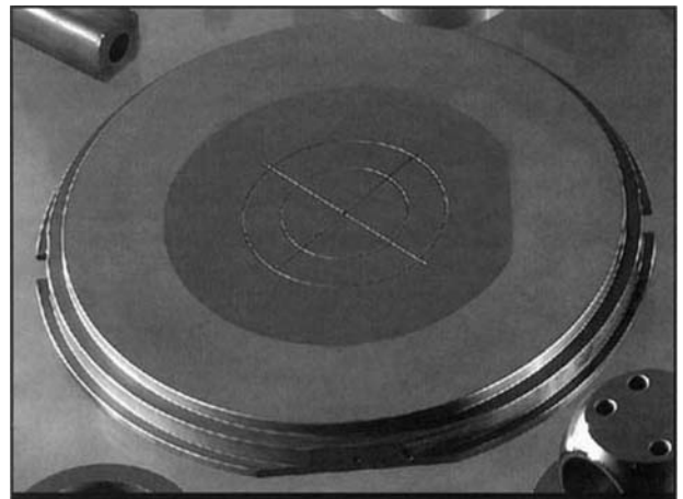
Figure 6-6. Vacuum chuck used to hold a silicon wafer in position during various high-temperature vapor deposition steps. Approximately 12 inches across, showing outline of position of silicon wafer. (Photo courtesy of Saint-Gobain/Carborundum Structural Ceramics, Niagara Falls, NY.)
