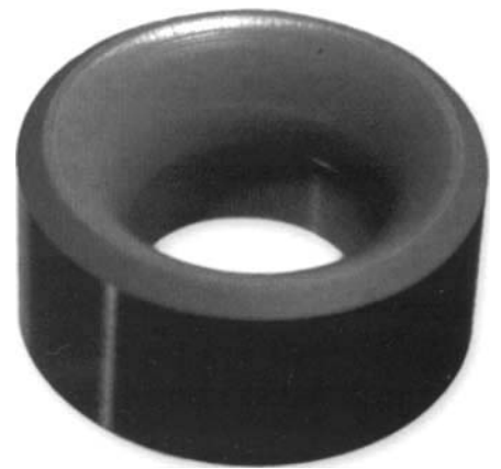
Figure 10-8. Zirconia die liner for hot extrusion of brass. (Photo by D. Richerson.)
