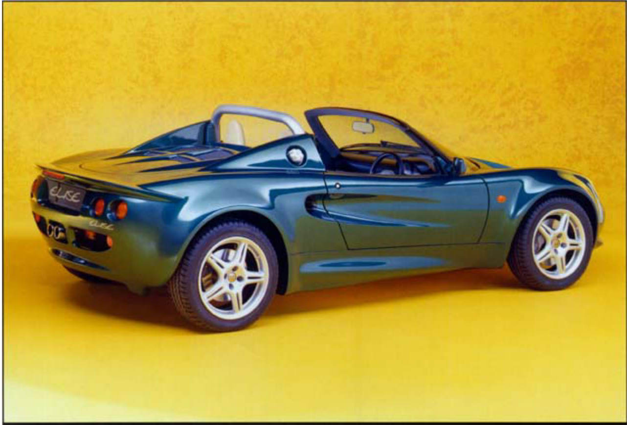
Figure 9-17. Lotus Elise automobile with the body constructed of glass-fiber-reinforced polymer and brake components fabricated from a Lanxide Automotive Company ceramic-metal composite. (Photo courtesy of Lotus Cars, Norfolk, England.)
