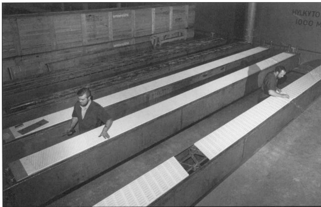
Figure 11-11.(top) View of ceramic foils and suction box covers installed on a paper machine. (Photo courtesy of Coors/Wilbanks, a Coors Company, Hillsboro, OR.)
