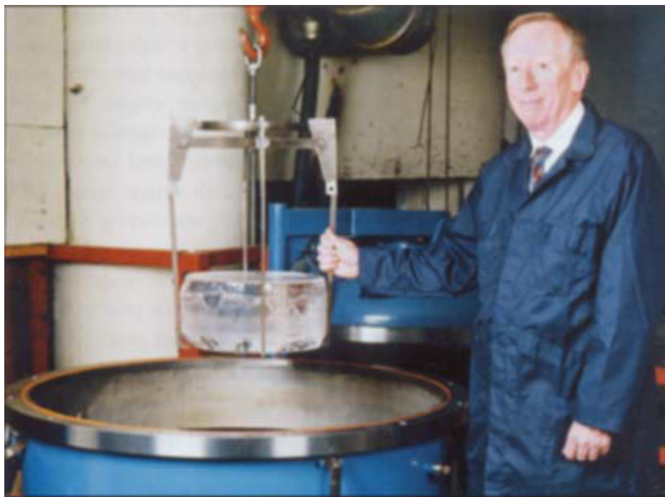
Figure 2-7. Enormous sapphire single crystal. This 13.4 inch diameter, 143 pound sapphire crystal was grown by the heat-exchanger process. (Courtesy of Crystal Systems, Inc., Salem, MA.)
