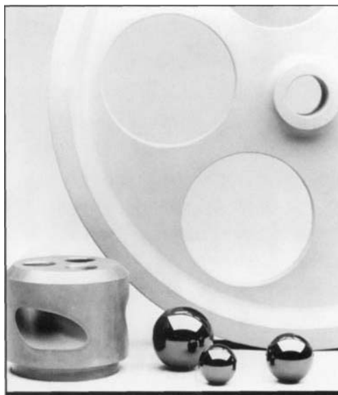
Figure 11-18. Silicon nitride ceramic parts for down-hole oil applications: sucker-rod balls, impulse rotor for a telemetry system, and an odometer wheel for down-hole measurements. (Photo courtesy of Ceradyne, Inc., Costa Mesa, CA.)
