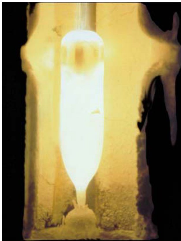
Figure 2-6. Single-crystal sapphire boule being “grown” by the Verneuil process. The colorless, clear boule will be cut into slices and ground and polished into watch faces for Rado watches; sapphire is much harder and more durable than glass and incredibly resistant to scratching. (Courtesy of the Rado Watch Co., Ltd., Lengnau, Switzerland.)
