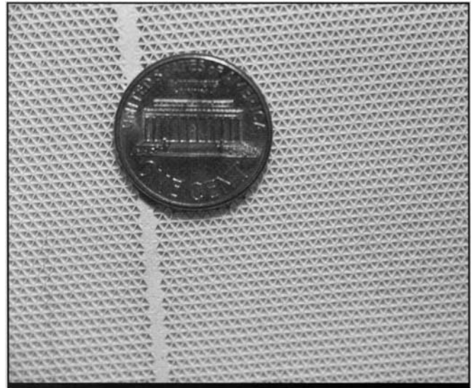
Figure 9-4. Close-up view of cordierite ceramic honeycomb. (Photo by D. Richerson.)
