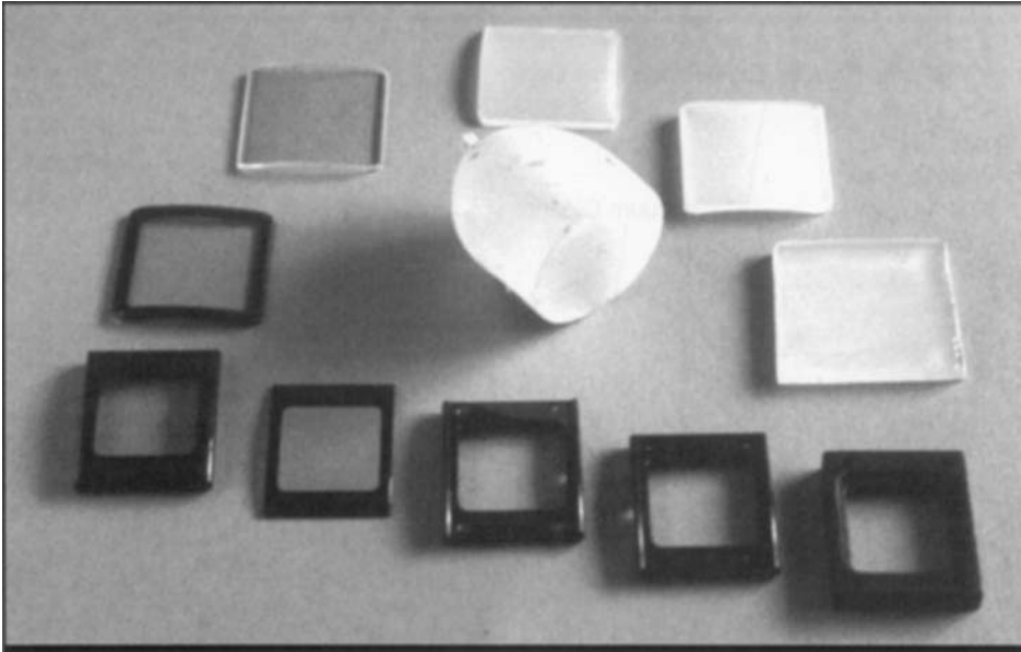
Figure 1-5. Steps in the fabrication of the watch glass and bezel of a Rado watch. (Samples courtesy of the Rado Watch Co., Ltd., photograph by D. Richerson.)
